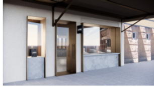
NEW GG-10 INTERNALLY ILLUMINATED BLAZE SIGNAGE CONICAL PIPES TO FACADE WALL CONCRETE: 400mm x 100mm x 400mm TEXT: LUNE - FINISH: BLACK STEEL BACKING, WHITE ILLUMINATED TEXT
